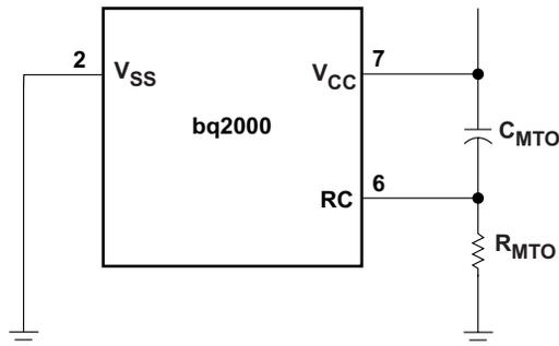
Figure 5. Typical Connection for the RC Input
