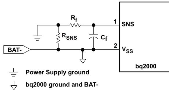
**Figure 9. Current-Sensing Circuit**
