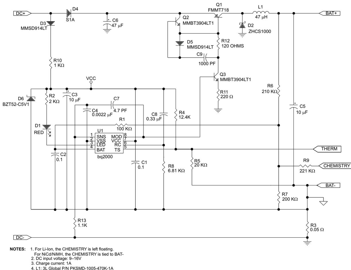
Figure 7. Single-Cell Li-Ion, 3-Cell NiCd/NiMH 1A Charger
