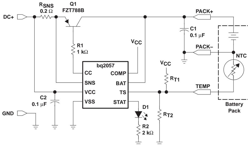
**Figure 1. Low Dropout Single- or Two-Cell Li-Ion/Li-Pol Charger**
