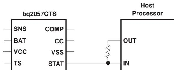
**Figure 11. Interfacing the bq2057 to a Host Processor**
