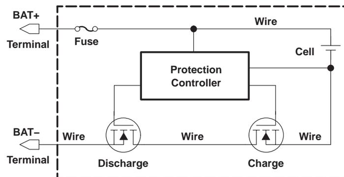
**Figure 12. Typical Components of a Single-Cell Li-Ion Pack**
