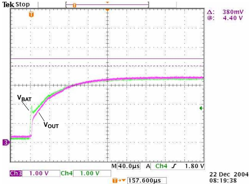
**Figure 12. Insert Battery – Power-Up Output via BAT**
