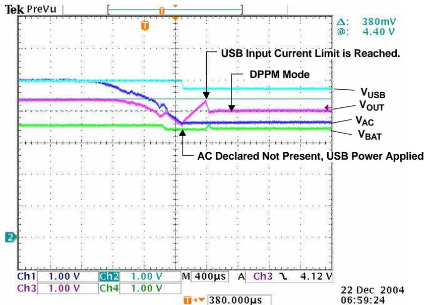
**Figure 7. Remove AC – PWR XFER to USB**
