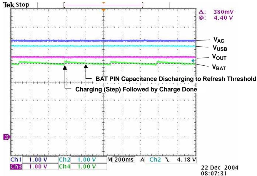
**Figure 11. Battery Absent – PWR XFER to USB**
