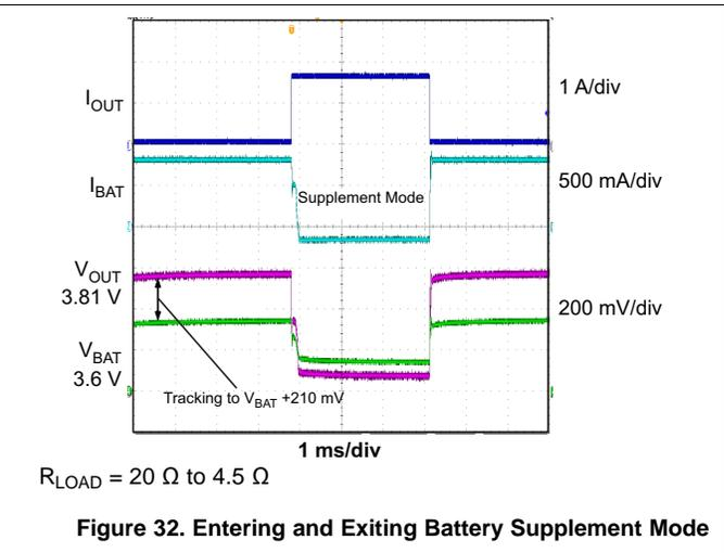
Figure 32. Entering and Exiting Battery Supplement Mode
