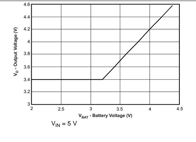
**Figure 4. bq24078 Output Regulation Voltage vs Battery Voltage**
