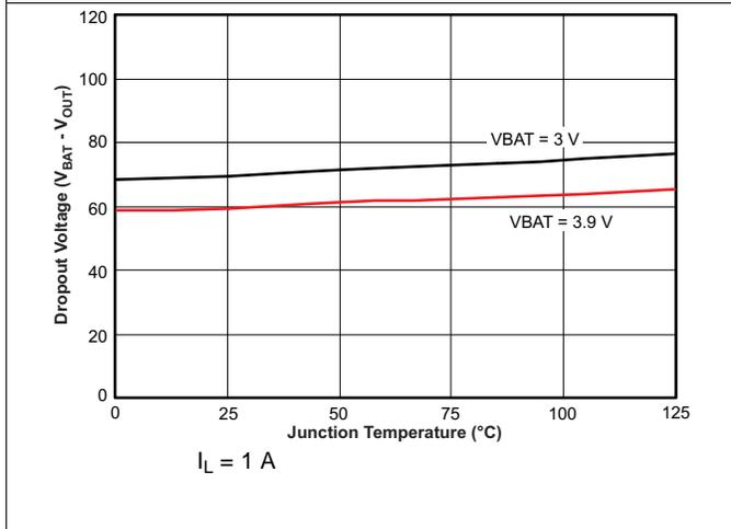
**Figure 3. Dropout Voltage vs Temperature No Input Supply**
