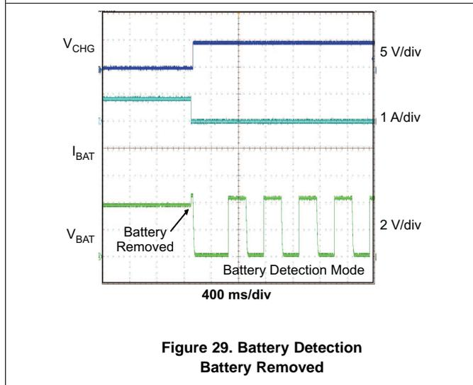
Figure 29. Battery Detection Battery Removed
