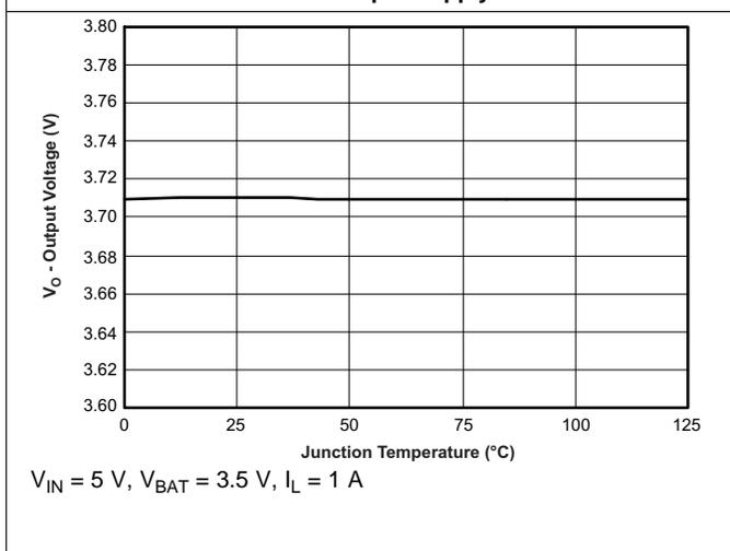
**Figure 5. bq24078 Output Regulation Voltage vs Temperature**
