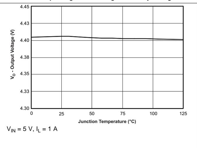
**Figure 6. bq24076 Output Regulation Voltage vs Temperature**
