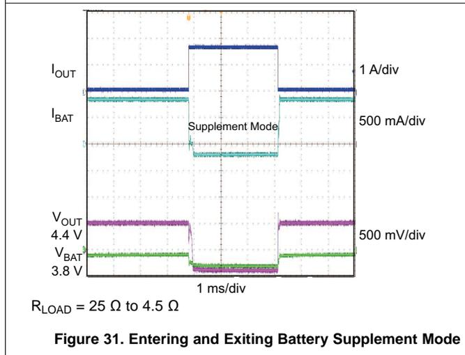
Figure 31. Entering and Exiting Battery Supplement Mode
