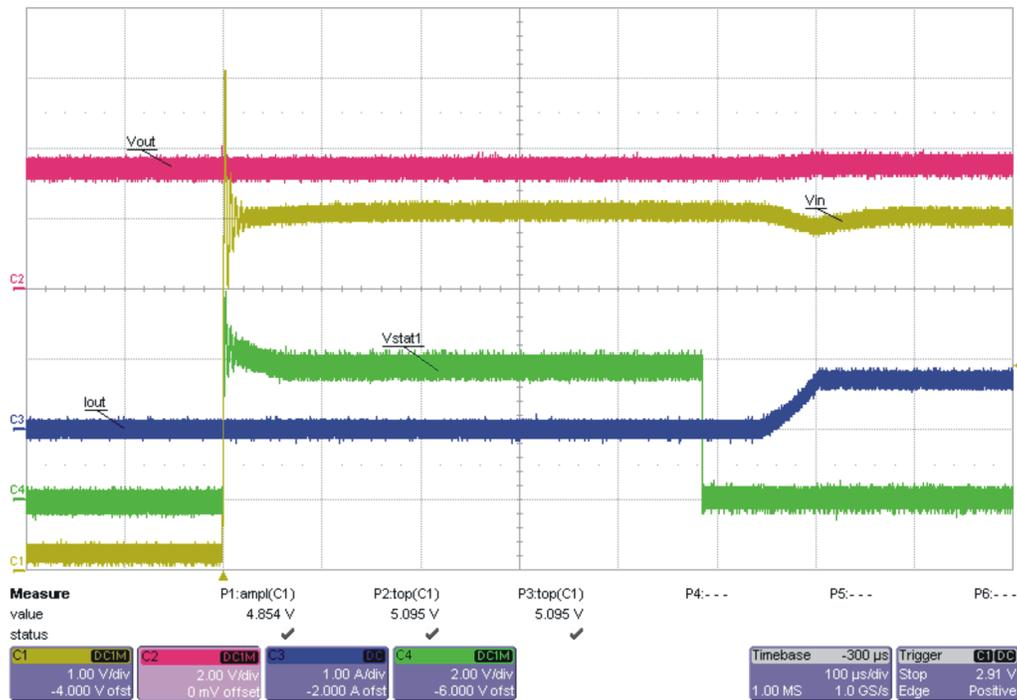
Figure 2. V<sub>IN</sub> Hot-Plug Power-Up Sequence
