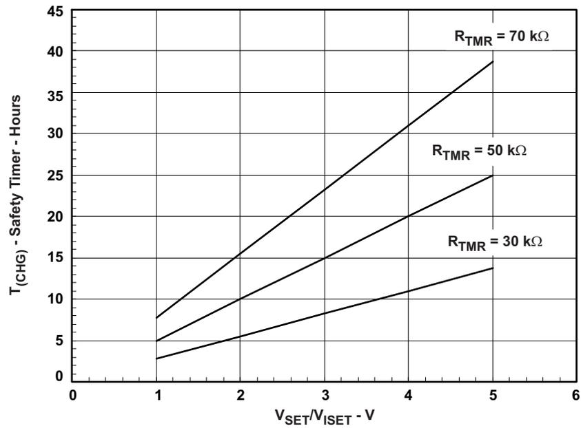
Figure 17. bq24085/6/78 Safety Timer Linearity for  $R_{TMR}$  Values
