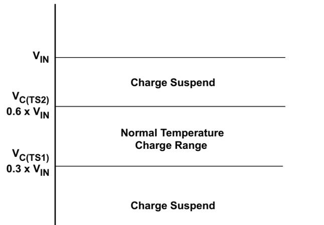
Figure 15. Battery Temperature Qualification With NTC Thermistor
