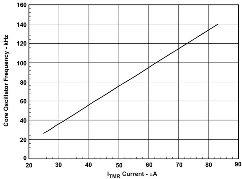
Figure 18. bq24085/6/7/8 Oscillator Linearity vs  $I_{TMR}$
