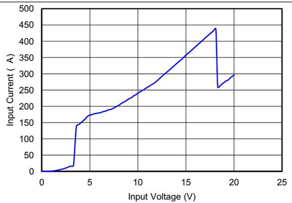
Figure 10. Input IQ with Charge Enable and Hi-Z
