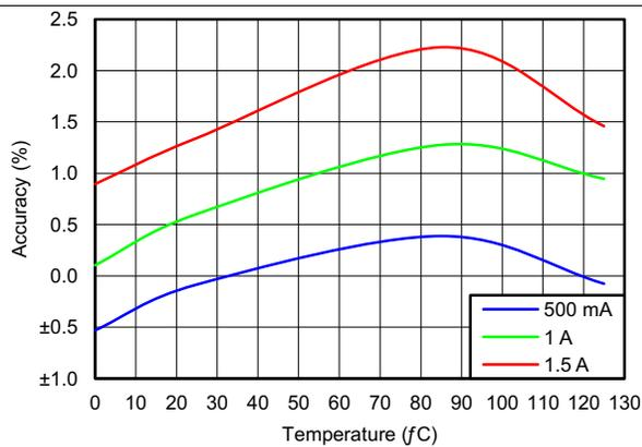
Figure 11. I<sub>CHG</sub> Accuracy with Internal Settings, V<sub>BAT</sub> = 3.3 V
