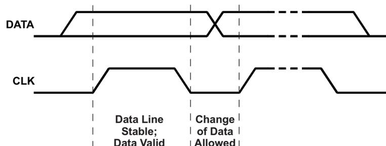
Figure 26. Bit Transfer on the Serial Interface
