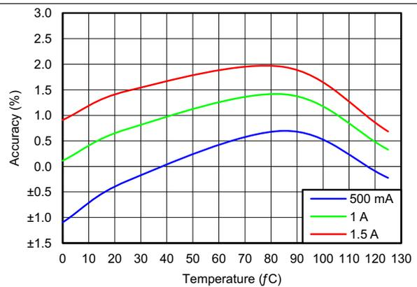
Figure 12. I<sub>CHG</sub> Accuracy with Internal Settings, V<sub>BAT</sub> = 3.8 V
