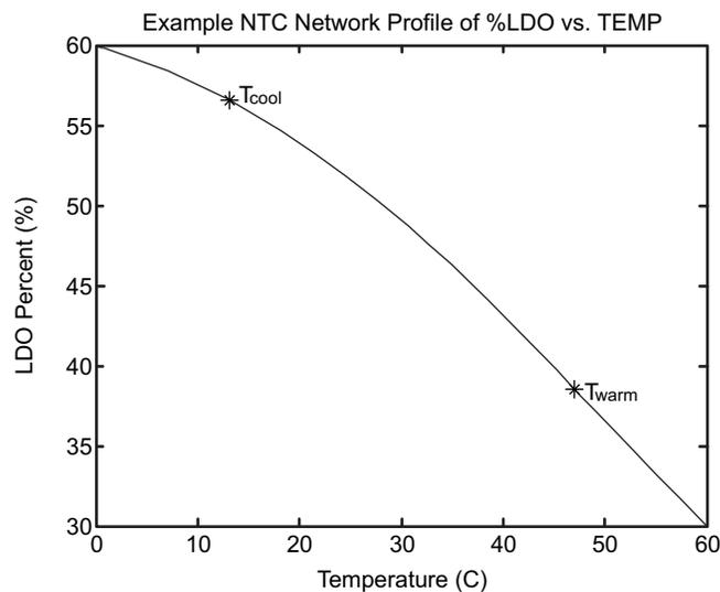
**Figure 22. Voltage Based NTC Circuit Temperature Profile**
