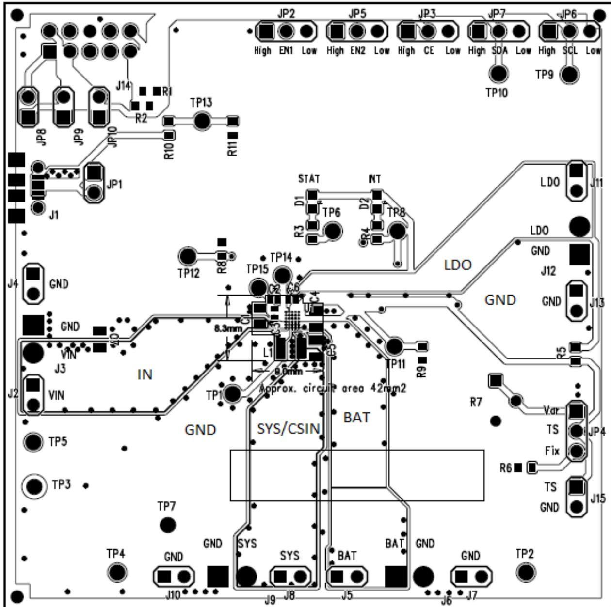
Figure 34. Recommended bq2425x PCB Layout for DSBGA Package
