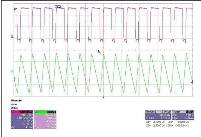
Figure 32. 1.0 μH CCM Operation
