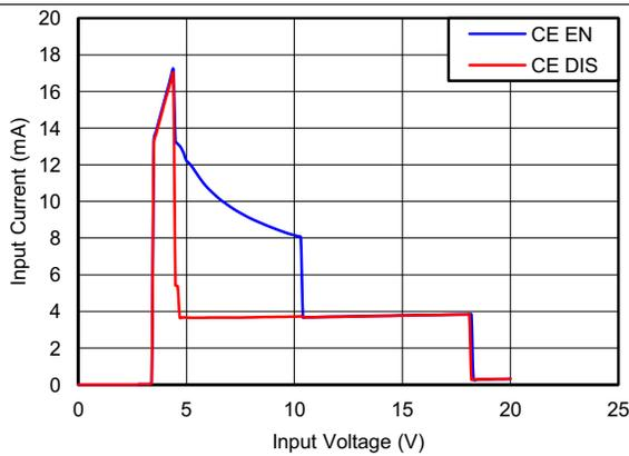
Figure 9. Input IQ With Charge DIS and EN
