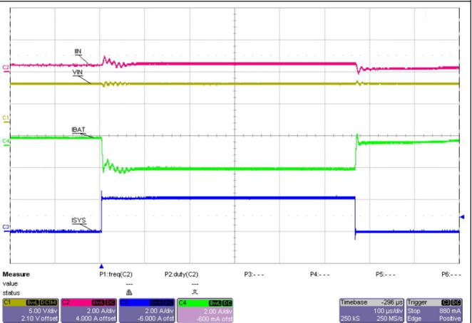
Figure 33. 2A Load Step Transient
