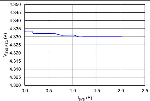
Figure 4. System Voltage Regulation vs Load Current
