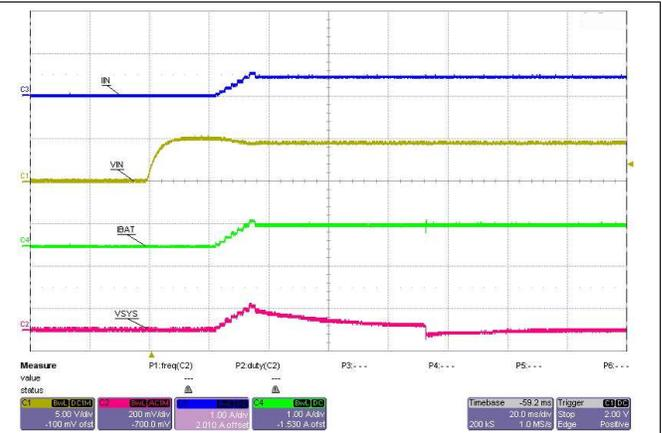
Figure 31. V<sub>DPM</sub> Startup, 4.2 V
