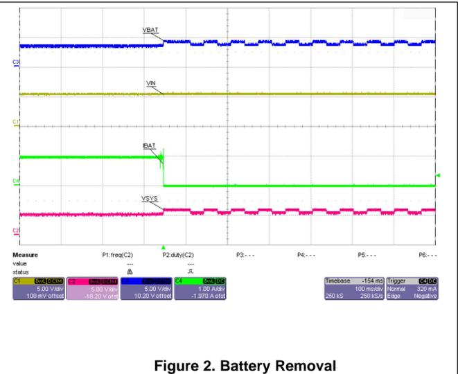
Figure 2. Battery Removal
