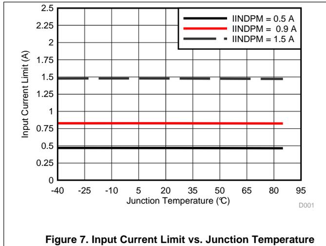
Figure 7. Input Current Limit vs. Junction Temperature
