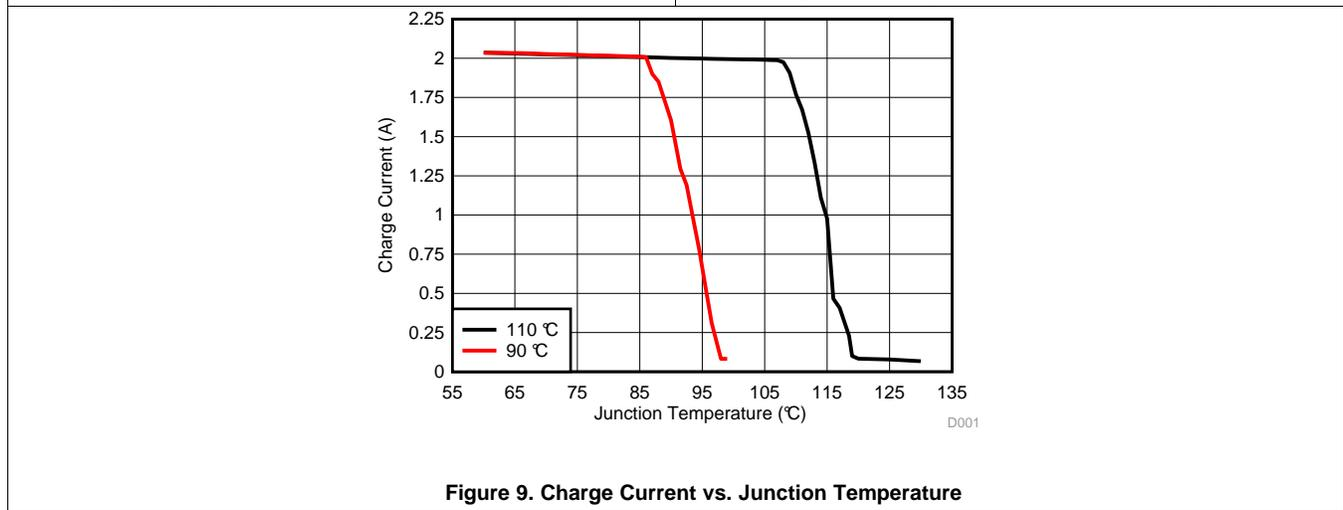
Figure 9. Charge Current vs. Junction Temperature
