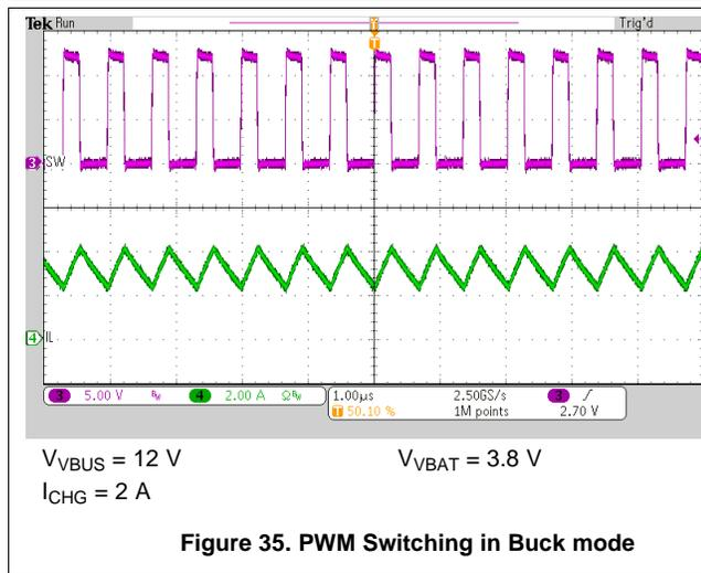
Figure 35. PWM Switching in Buck mode
