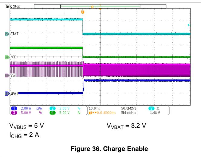
Figure 36. Charge Enable
