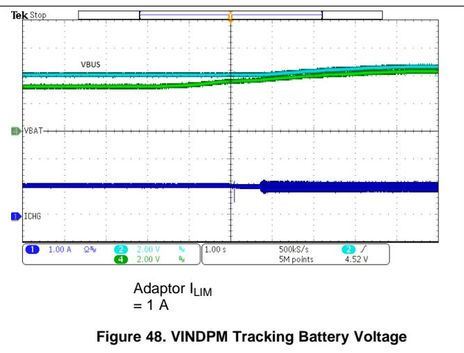
Figure 48. VINDPM Tracking Battery Voltage
