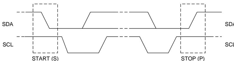
Figure 21. TS START and STOP conditions
