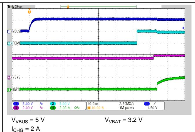
Figure 30. Power-Up with Charge Enabled
