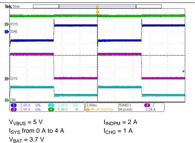
Figure 42. System Load Transient
