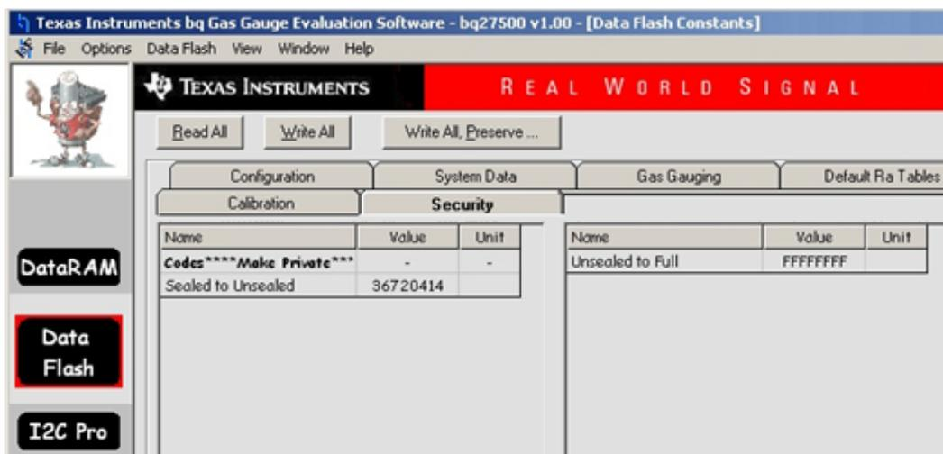
Figure 23. Sealed Mode for the bqEVS DataRAM window
