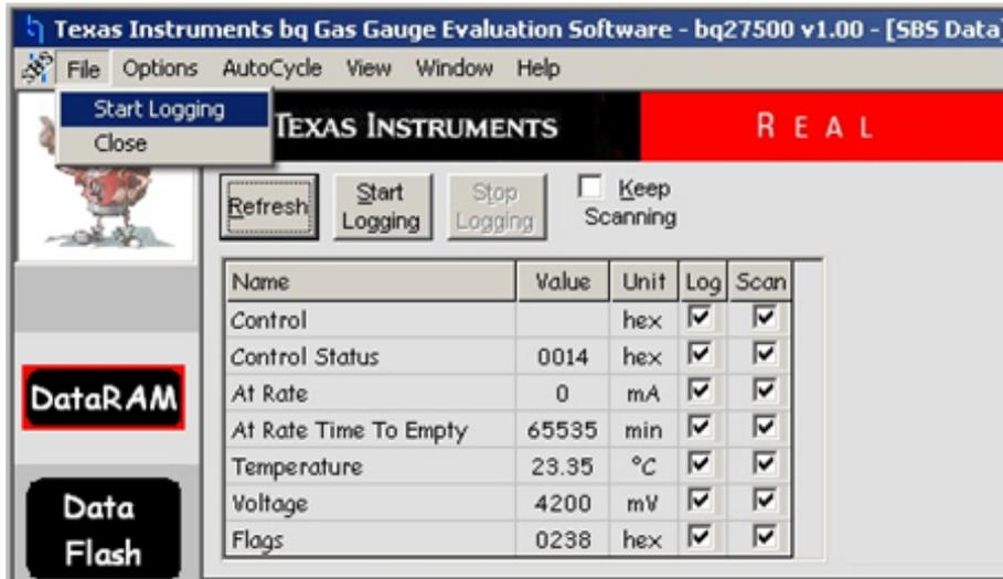
To save the iterations of the Gas Gauge (.GG) file, go to the **Data Flash** window and select the **Options** → **Set AutoExport Filename** command. A series of Gas Gauge files is created in the folder specified throughout the testing. You can adjust the save interval of AutoExport (every 15 minutes is usually acceptable) using the **Options** → **Set Export Interval** command. To start the logging, select the **Options** → **AutoExport** command (Figure 21) to begin saving the Gas Gauge files.
