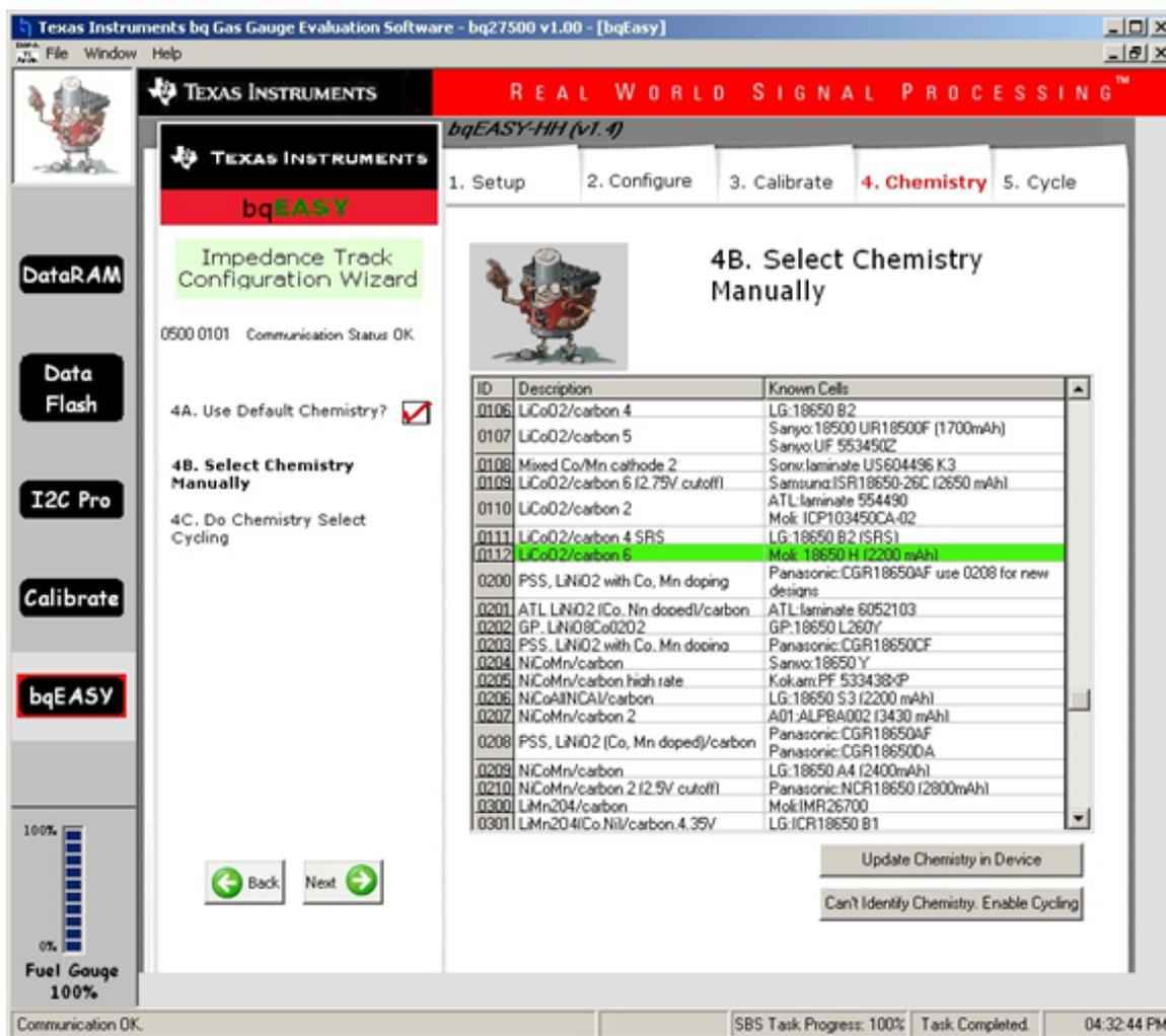
A unique chemical ID indicates a different battery chemistry being used.
