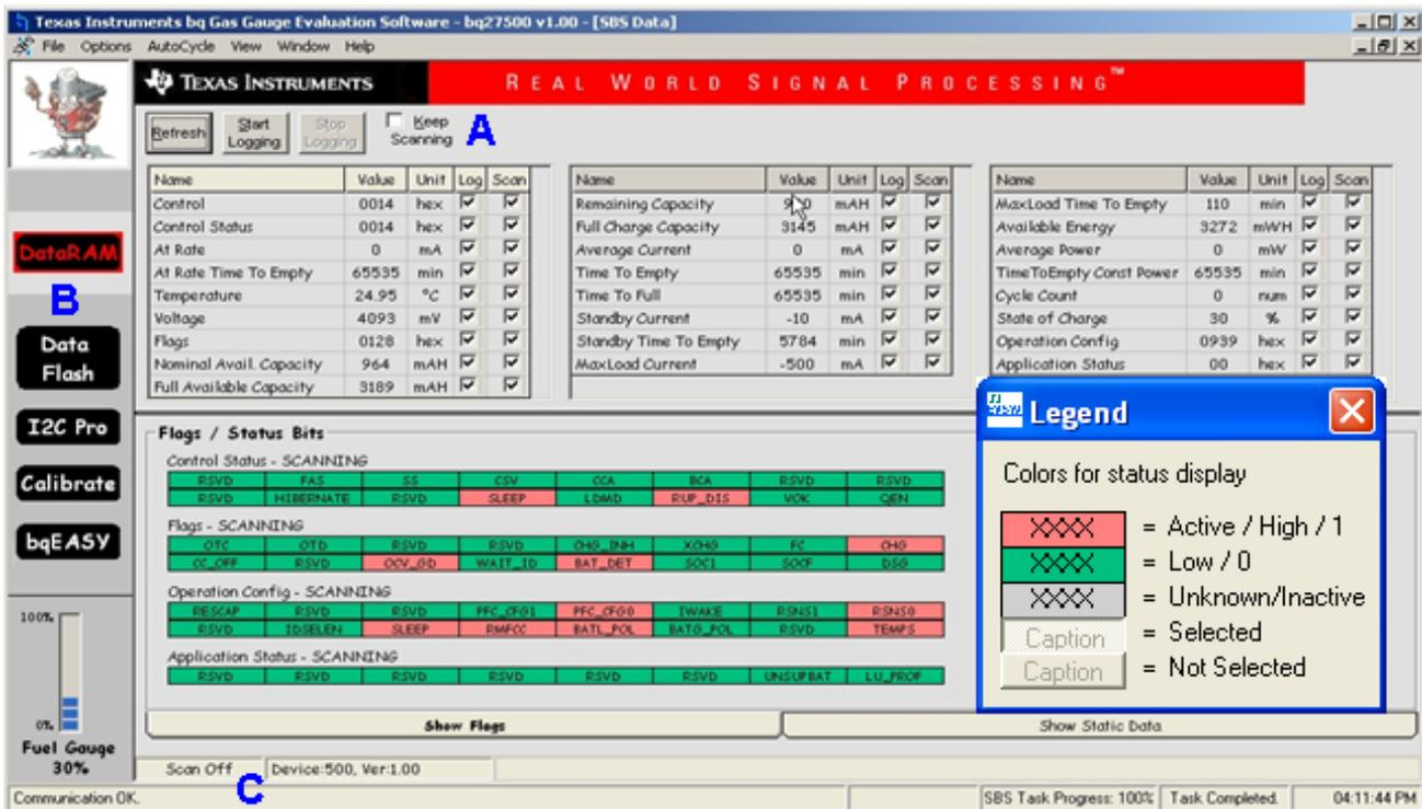
You can issue Manufacture Access commands (MAC) from this window by clicking in the **Control** field under the *Value* column (see [Issuing MACs procedures](#)). For example, this issue arises when writing the Unseal or Full Access commands. Examples of how to complete these processes is included in [Seal and Unseal Process](#).
