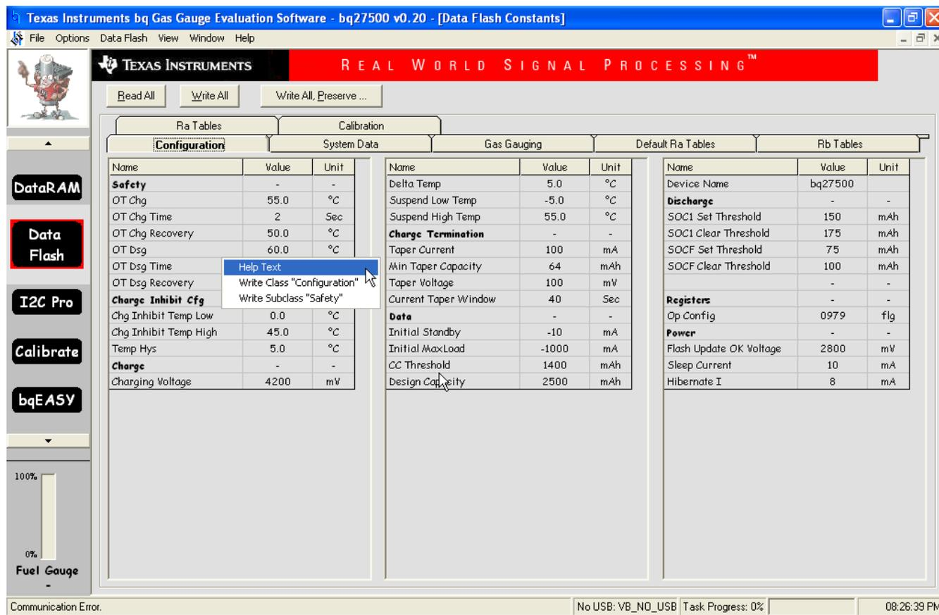
Remembering all the nuances of the Data Flash parameters is not practical. However, all of the Data Flash definitions are listed in the *bq2750x Technical Reference Manual*. Additionally, you can right-click on any Data Flash parameter and choose *Help Text* (Figure 12), which displays an appropriate definition.
