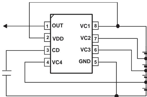
Figure 1.  $I_{CC}$ ,  $I_{IN}$  Measurement (DCT Package)
