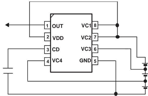
Figure 4. 3-Series Cell Configuration
