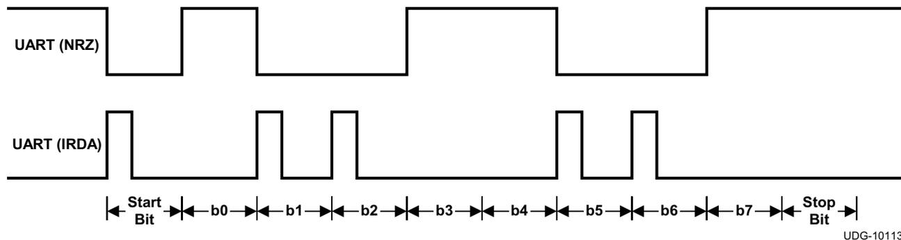
Figure 4. UART Encoding
