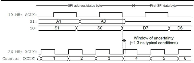
SPI Read Synchronization Issue — SPI read synchronization results in incorrect read values for register fields that are continuously updated www.ti.com
