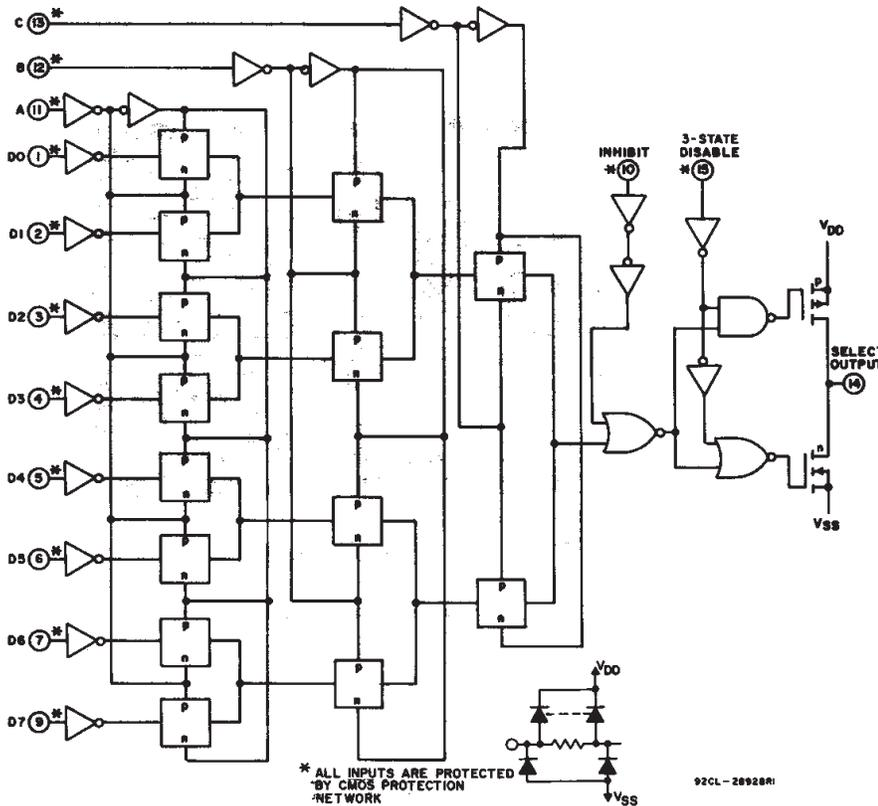
Fig. 1 - Logic diagram.
