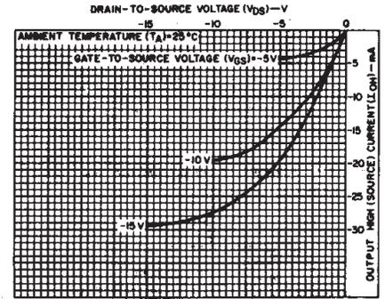
Fig. 5 - Typical output high (source) current characteristics.
