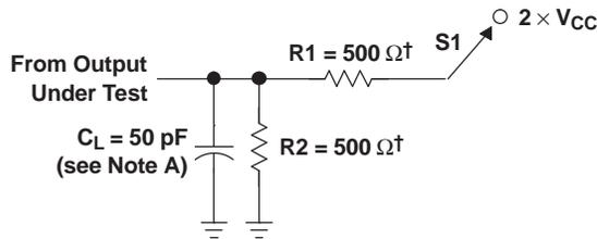
$^\dagger$  When  $V_{CC} = 1.5\text{ V}$ ,  $R_1 = R_2 = 1\text{ k}\Omega$
