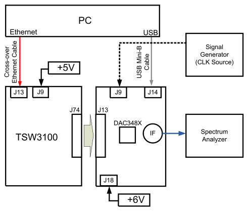
Figure 16. Test Setup Block Diagram for TSW3100
