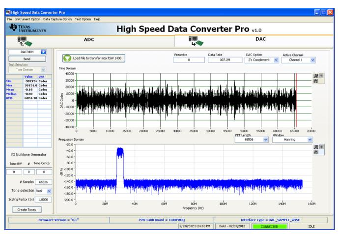
Figure 12. Load File to Transfer into TSW1400
