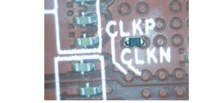
Figure 15. TSW3100 FPGA Clock 100-Ω LVDS Termination at Pins T31 and T32 of the FPGA
