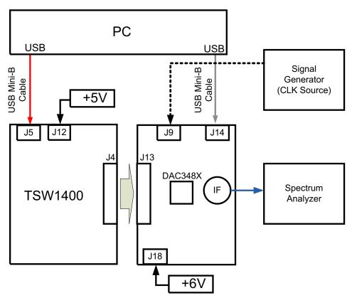
Figure 8. Test Setup Block Diagram for TSW1400
