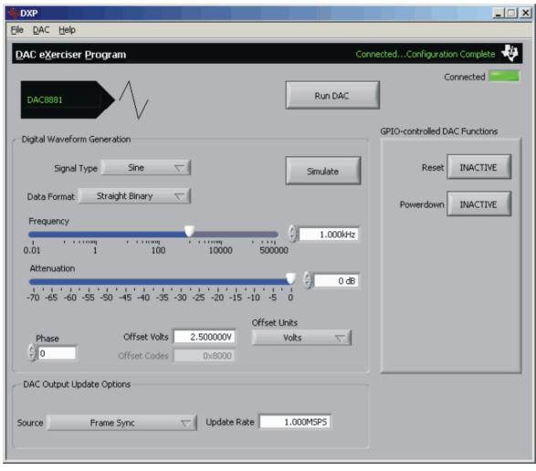
Figure 13. DAC8881 - Frequency/Amplitude and GPIO Control Options
