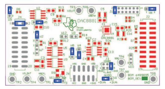
Figure 10. DAC8881 EVM Default Jumper Configuration
