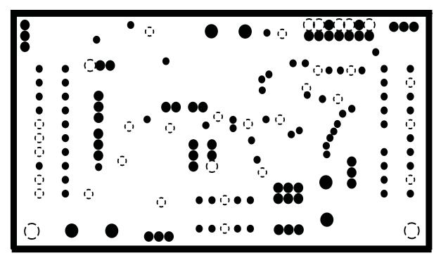
Figure 4. Layer 2 (Ground Plane)
