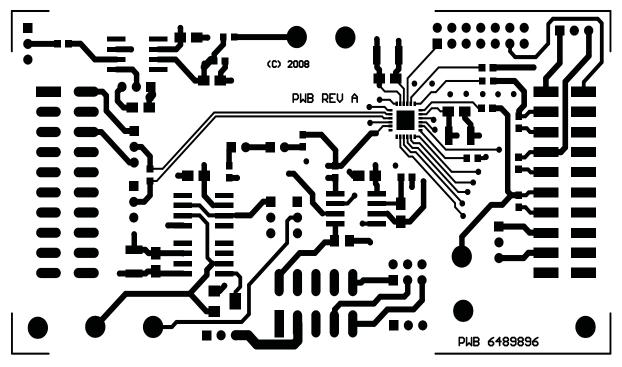
Figure 3. Layer 1 (Top Signal Plane)
