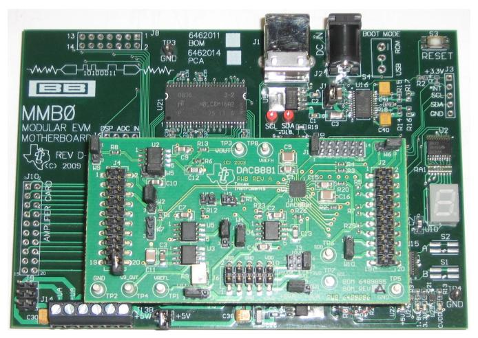
Figure 11. MMB0 with DAC8881EVM Installed
