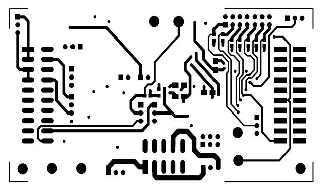
Figure 6. Layer 4 (Bottom Signal Plane)
