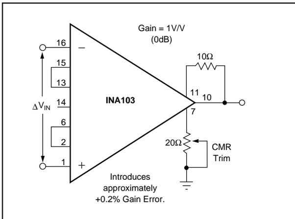
FIGURE 10. Optional Circuit for Externally Trimming CMR.
