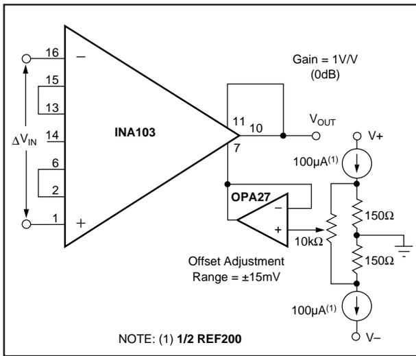
FIGURE 4. Output Offsetting.
