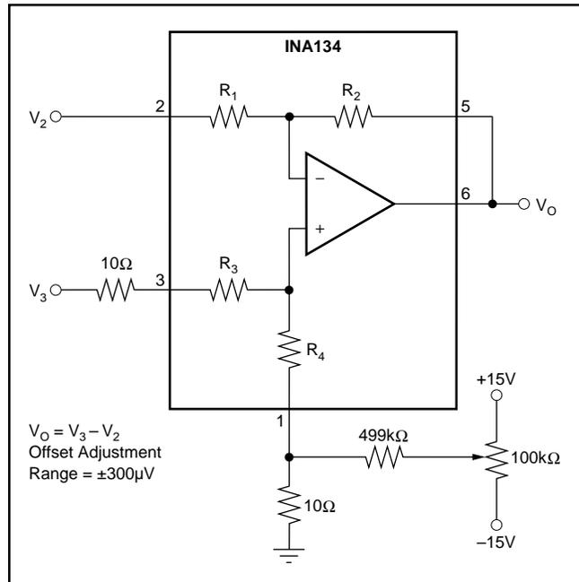
FIGURE 2. Offset Adjustment.
