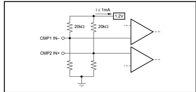
Figure 37. Limit Current Into Reference  $\leq 1mA$
