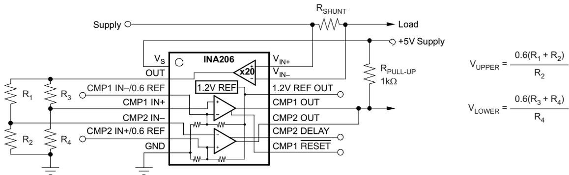
$$V_{\text{UPPER}} = \frac{0.6(R_1 + R_2)}{R_2}$$
