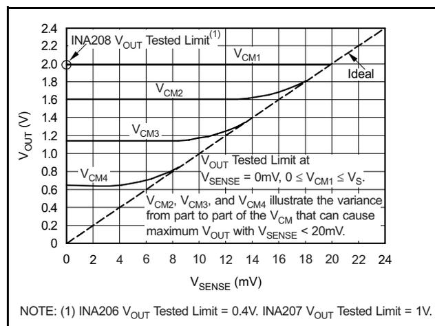
**Figure 32. Example for Low  $V_{SENSE}$  Case 2 (INA208, Gain = 100)**
