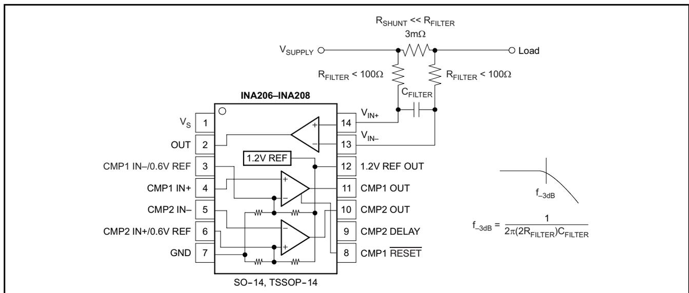
Figure 33. Input Filter (Gain Error  $-1.5\%$  to  $-2.2\%$ )
