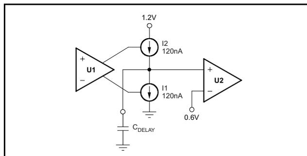
Figure 34. Simplified Model of the Comparator 2 Delay Circuit
