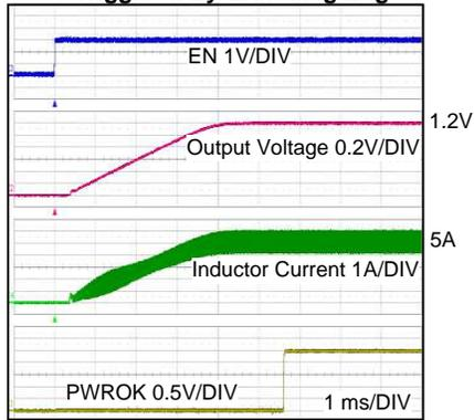
**Soft Start With 0.5V Pre-bias Voltage, DCM Operation, Triggered By PWI 'Wakeup' Command**
