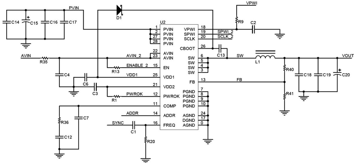
Figure 10. LM10500 Evaluation Board Schematic (Part I)
