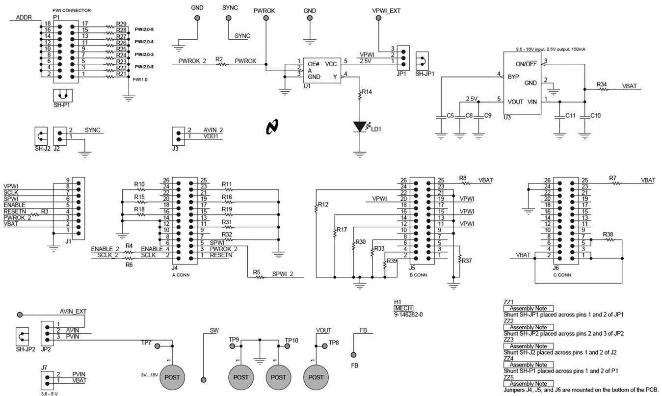
Figure 11. LM10500 Evaluation Board Schematic (Part II)
