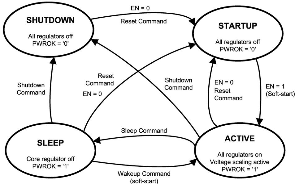
**Figure 7. PWI Slave Operation States Diagram**
