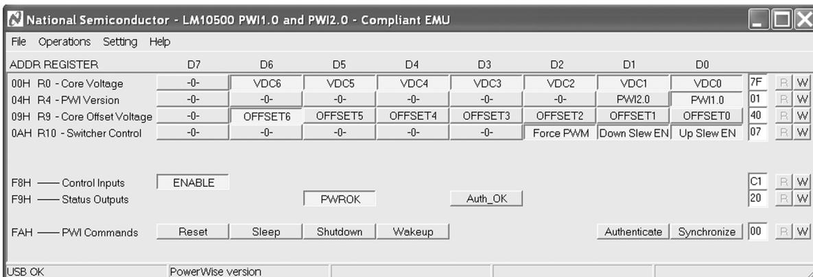
**Figure 6. The LM10500 GUI With Default Register Values And Status (LM10500SQ-0.8)**
