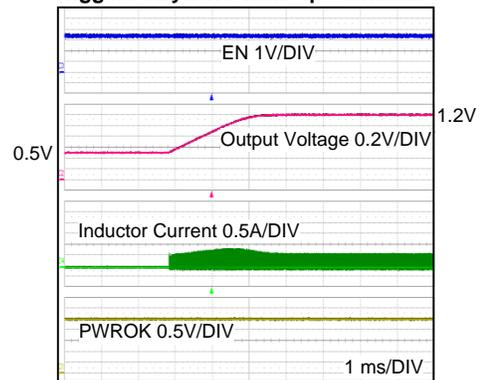
**Soft Start With 0.5V Pre-bias Voltage, CCM Operation, Triggered By PWI 'Wakeup' Command**
