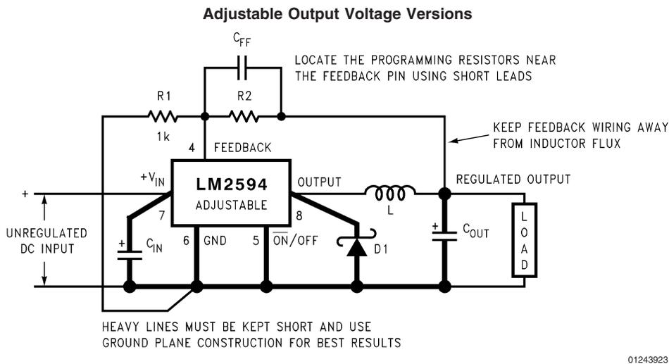
$$V_{OUT} = V_{REF} \left( 1 + \frac{R_2}{R_1} \right) \quad \text{where } V_{REF} = 1.23V$$
