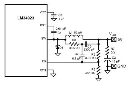
Figure 4. Minimum Output Ripple Configuration
