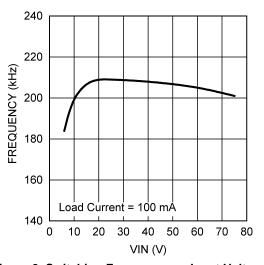
Figure 8. Switching Frequency vs. Input Voltage
