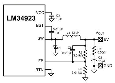
Figure 3. Reduced Ripple Configuration
