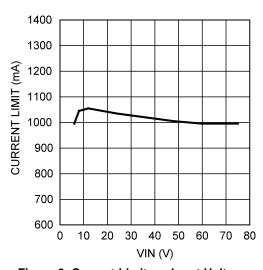
Figure 9. Current Limit vs. Input Voltage
