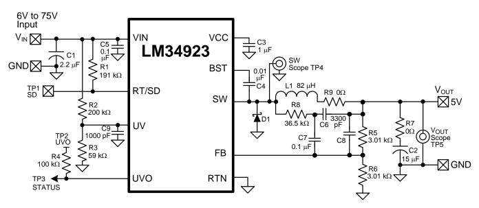
Figure 6. Complete Evaluation Board Schematic (As Supplied)
