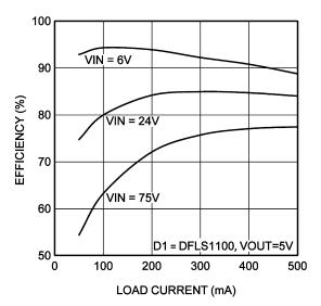
Figure 5. Efficiency at 200 kHz
