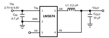
Figure 1. Typical Application Circuit: Fixed Voltage
