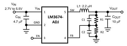
Figure 2. Typical Application Circuit: Adjustable Voltage
