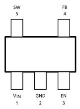
Figure 3. SOT23-5 Package, Top View
