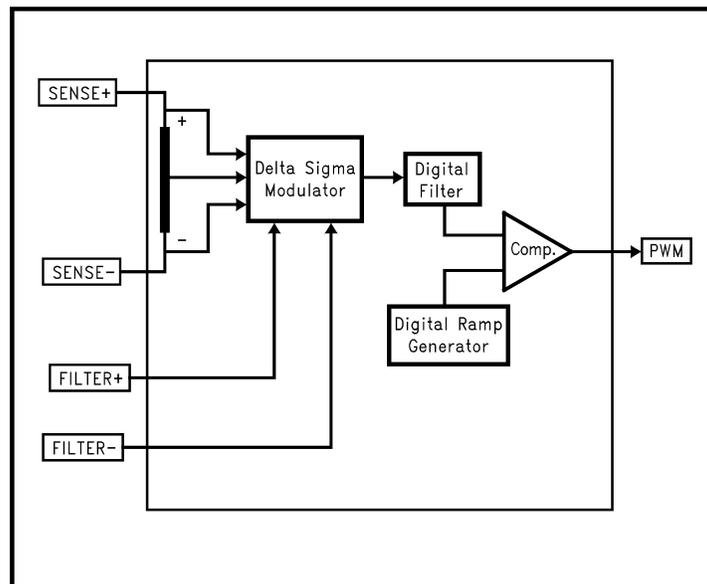
Figure 22. Functional Block Diagram of LM3812 and LM3813
