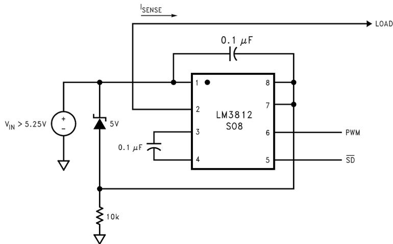
**Figure 20. High Voltage Operation —  $V_{IN}$  Greater Than 5.25V (High Side Sense)
