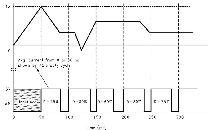
Duty cycle of the PWM waveform during any sampling interval indicates the current magnitude (average) and direction during the previous sampling interval.
