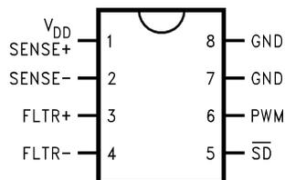
**Figure 1. LM3812 (Top View) for High-Side Sensing**
