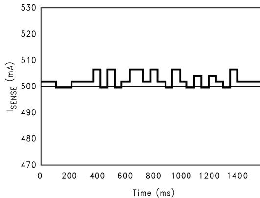
Figure 24. Typical Response of LM3812-1.0/LM3813-1.0
