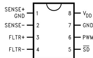
**Figure 2. LM3813 (Top View) for Low-Side Sensing**
