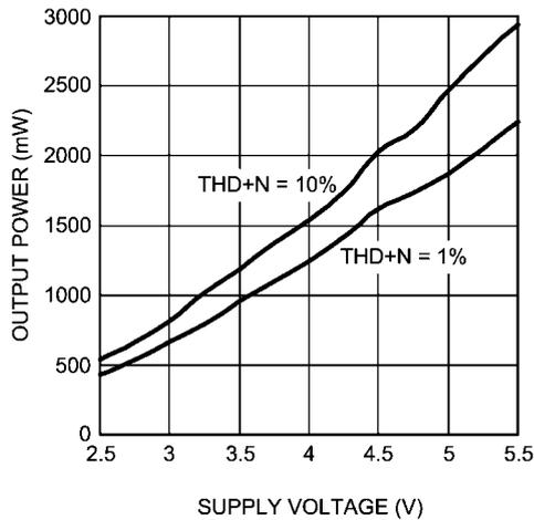
**Output Power/channel vs Supply Voltage**
