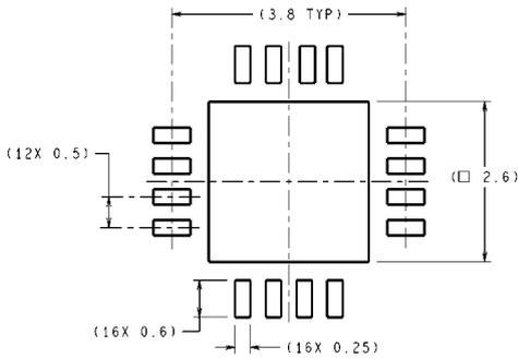
DIMENSIONS ARE IN MILLIMETERS
