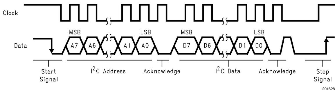
FIGURE 3. I<sup>2</sup>C Bus Format
