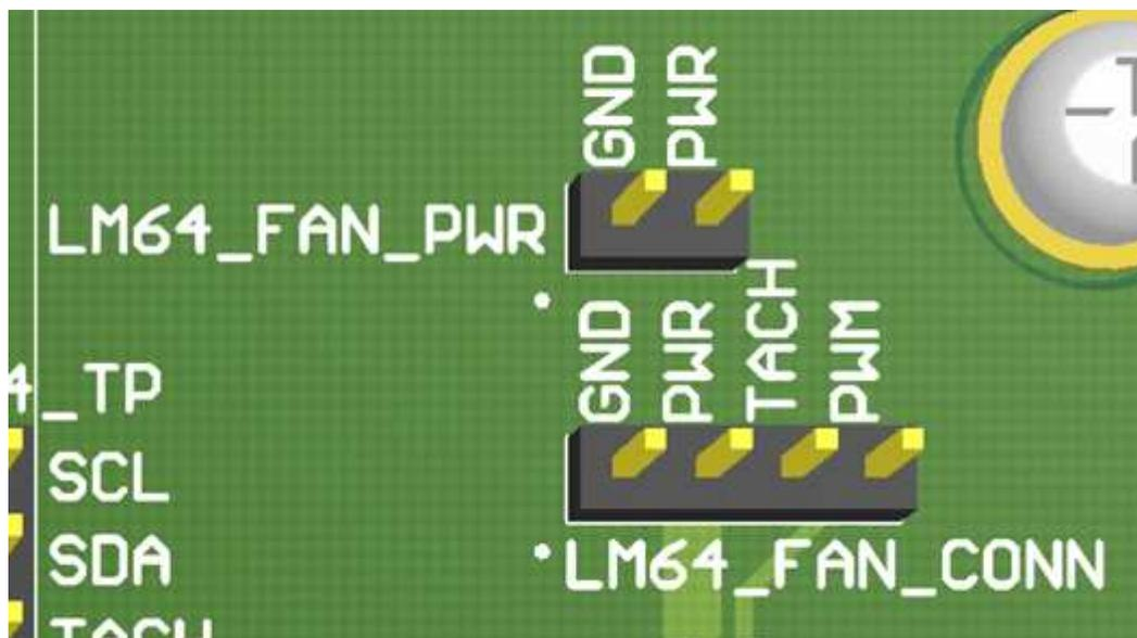
Figure 15. LM64 Fan Connector
