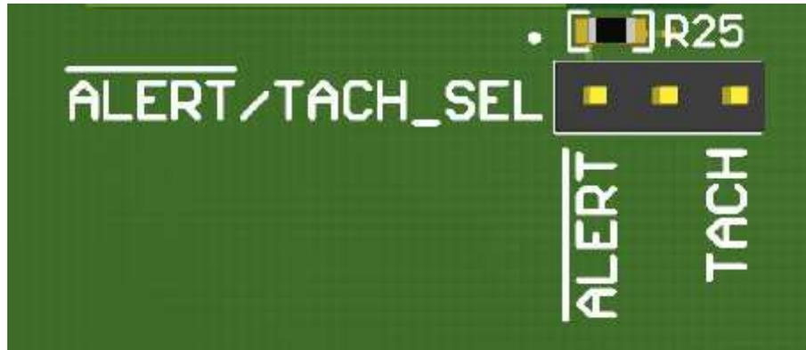
Figure 4. LM63 ALERT/TACH Select Jumper
