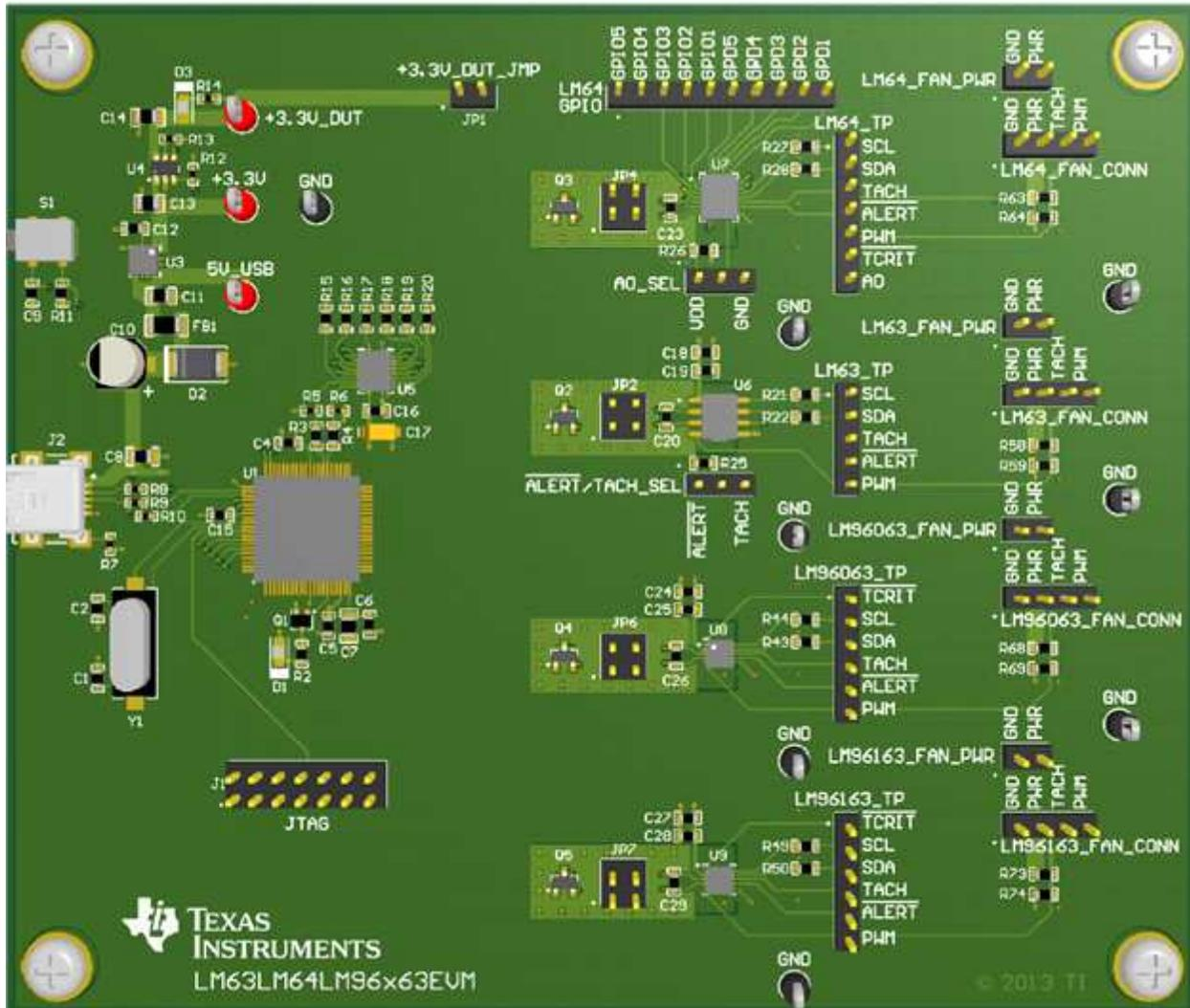
Figure 1. LM63LM64LM96x63EVM Board
