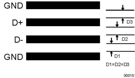
FIGURE 9. Ideal Diode Trace Layout
