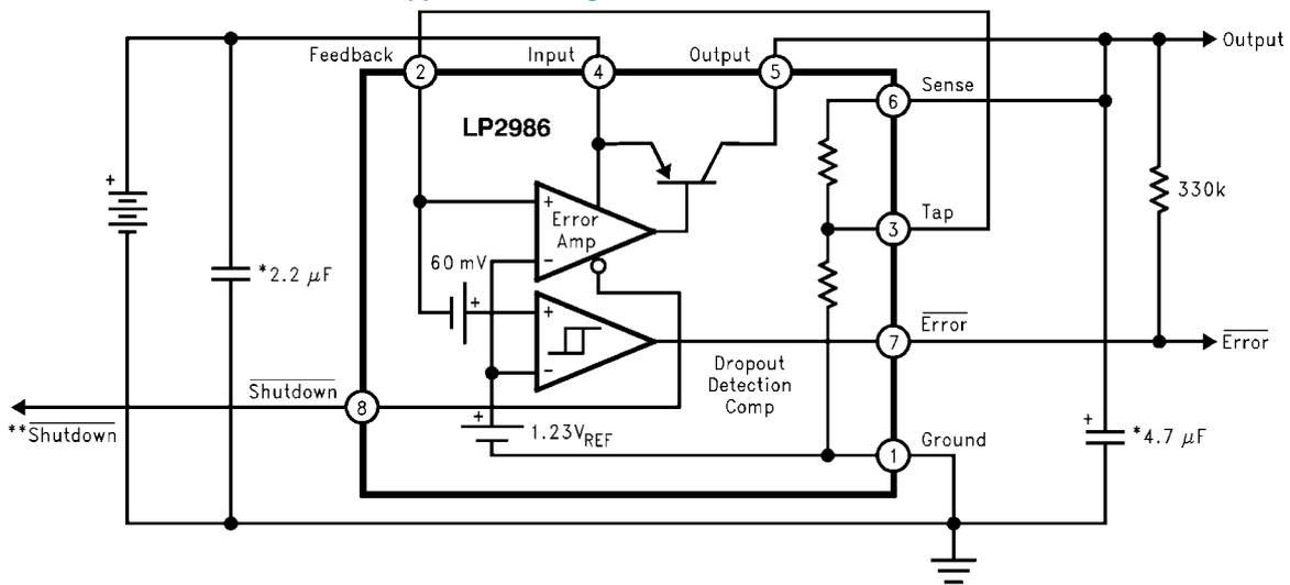
\* Minimum capacitance shown to assure stability, but may be increased without limit. Larger output capacitor provides improved dynamic response.
