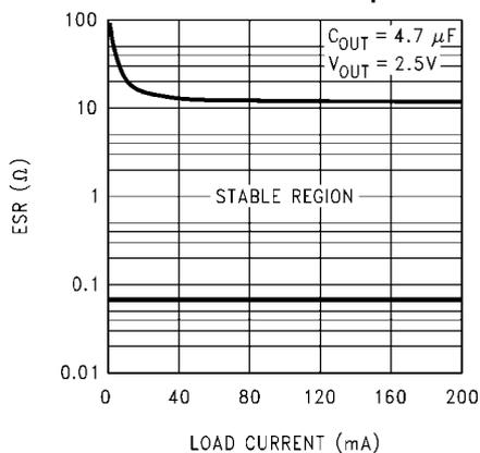
**IMPORTANT:** The output capacitor must maintain its ESR in the stable region over the full operating temperature range of the application to assure stability.
