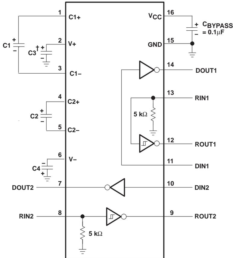
† C3 can be connected to VCC or GND.
