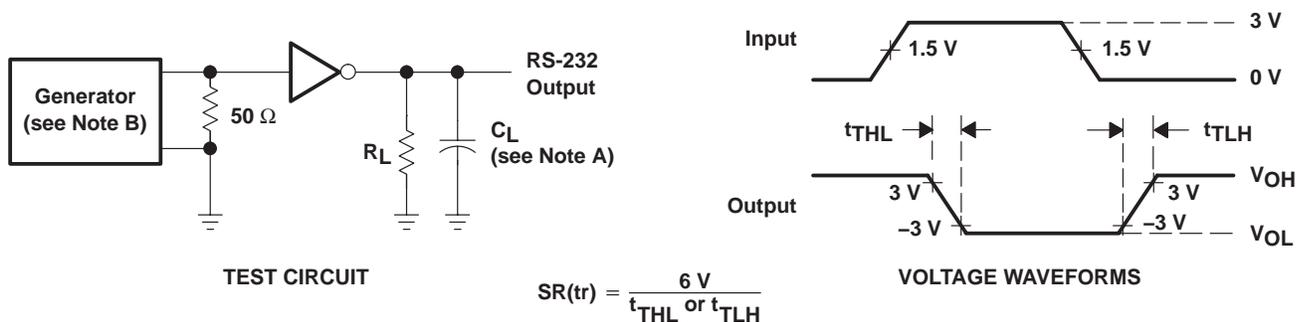
NOTES: A. C<sub>L</sub> includes probe and jig capacitance.
