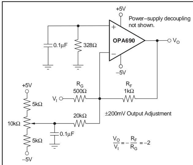
Figure 12. DC-Coupled, Inverting Gain of -2, with Offset Adjustment
