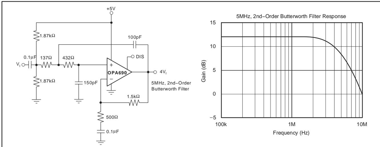
Figure 7. Single-Supply, High-Frequency Active Filter
