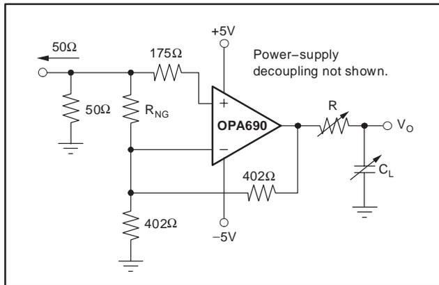
Figure 9. Capacitive Load Driving with Noise Gain Tuning
