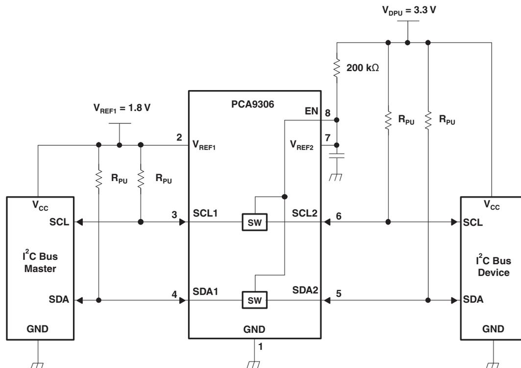
Figure 7. Typical Application Circuit (Switch Always Enabled)
