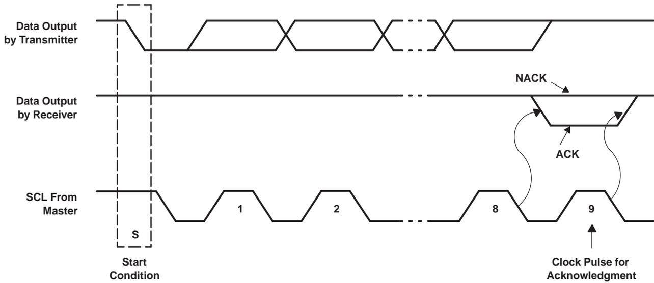
**Figure 3. Acknowledgment on I<sup>2</sup>C Bus**
