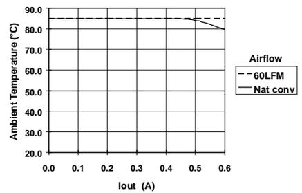
Note A: All Characteristic data in the above graphs has been developed from actual products tested at 25°C. This data is considered typical data for the converter.
