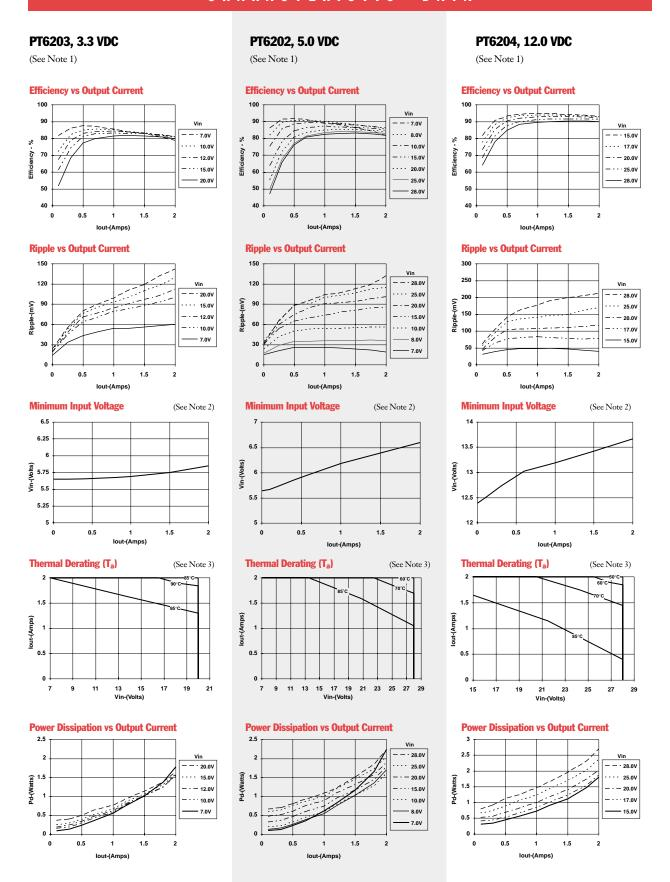
Note 1: All data listed in the above graphs, except for derating data, has been developed from actual products tested at 25°C. This data is considered typical data for the ISR.
