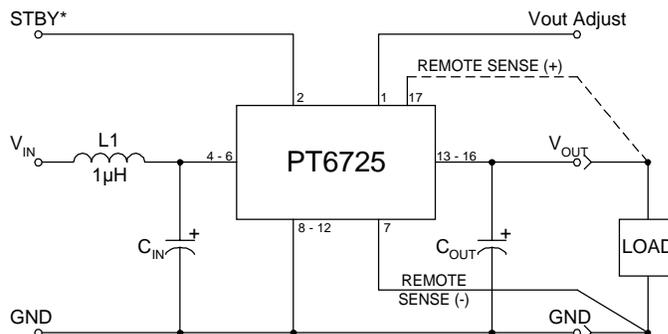
$C_{in}$  = Required 1000 $\mu$ F electrolytic
