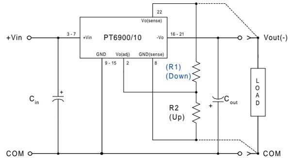
The respective values of (R1) [adjust down], and R2 [adjust up], can also be calculated using the following formulas.
