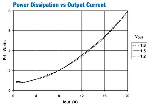
**Note A:** All characteristic data in the above graphs has been developed from actual products tested at 25°C. This data is considered typical for the ISR.
