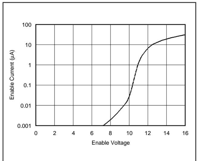
FIGURE 5. ENABLE Pin Current versus Applied Voltage.
