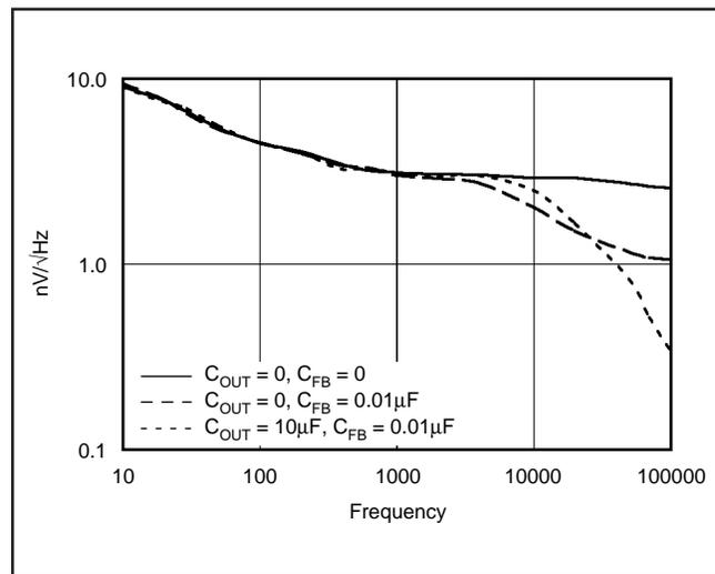
FIGURE 9. Output Noise Density on Adjustable Versions.
