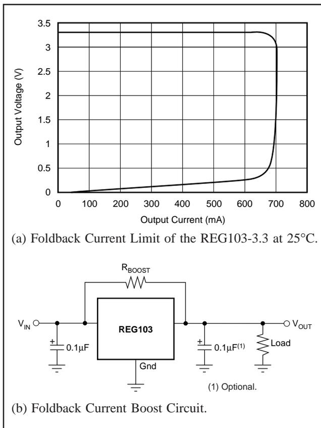
FIGURE 3. Foldback Current Limit and Boost Circuit.
