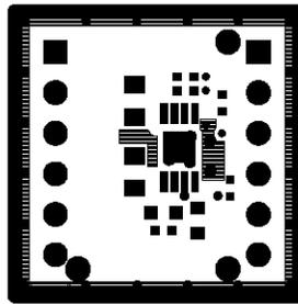
Figure 8. SMP-TPS7A3001-MVK Board Solder Mask – Top Side
