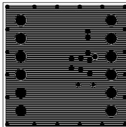
Figure 5. SMP-TPS7A3001-MVK Board Layer 2 – Ground Plane
