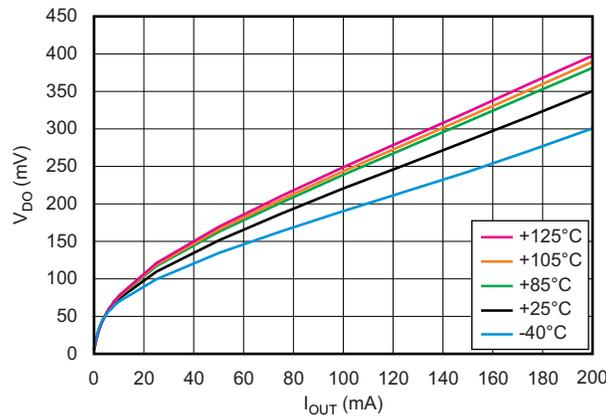
**Figure 3. TPS7A3001 Dropout Voltage Versus Output Current**
