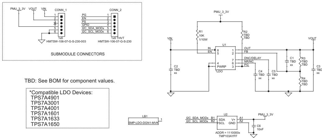
Figure 14. SMP-TPS7A3001-MVK Schematic
