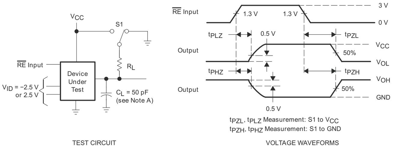
Figure 6. Receiver Test Circuit and Voltage Waveforms
