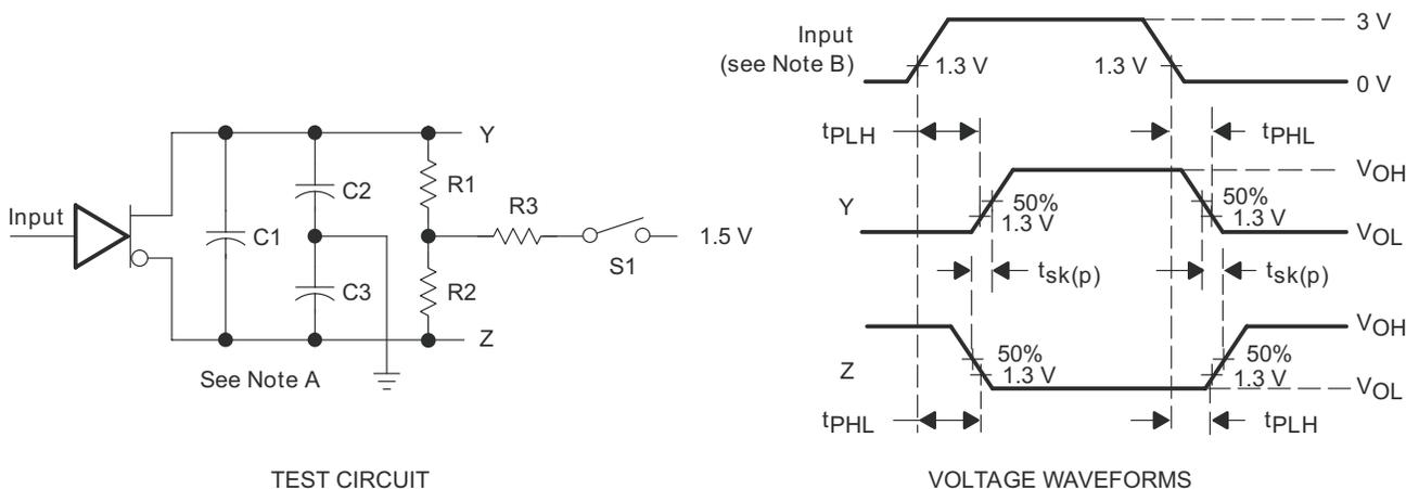
Figure 2. Driver Test Circuit and Voltage Waveforms
