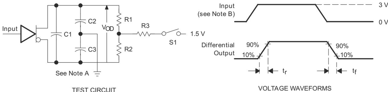
Figure 3. Driver Test Circuit and Voltage Waveforms
