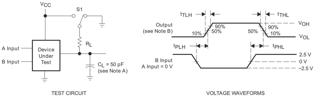
Figure 5. Receiver Test Circuit and Voltage Waveforms
