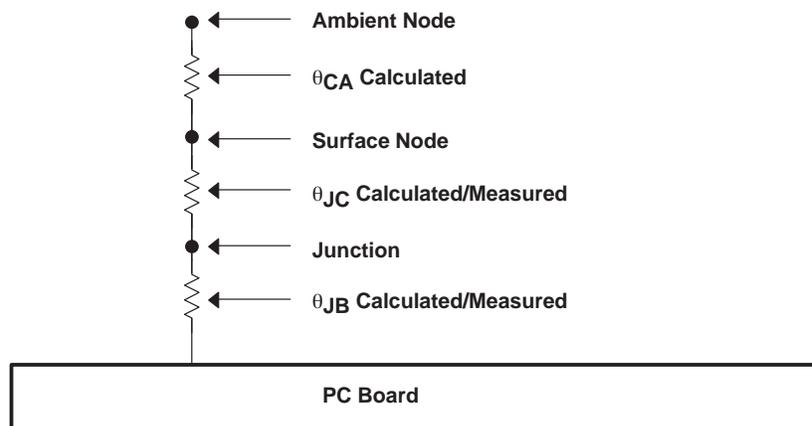
**Figure 12. Thermal Resistance**
