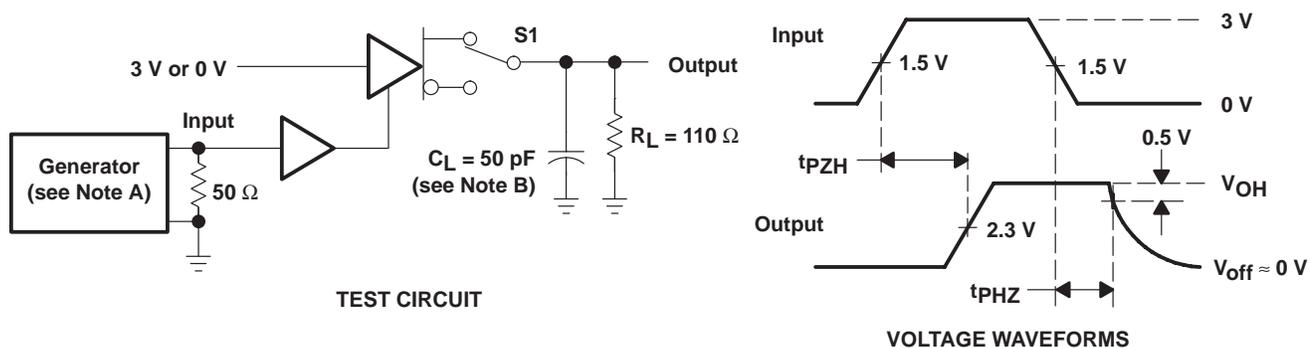
Figure 4.  $t_{pZH}$  and  $t_{pHZ}$  Test Circuit and Waveforms
