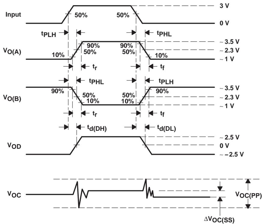
**Figure 5. Driver Timing, Voltage and Current Waveforms**
