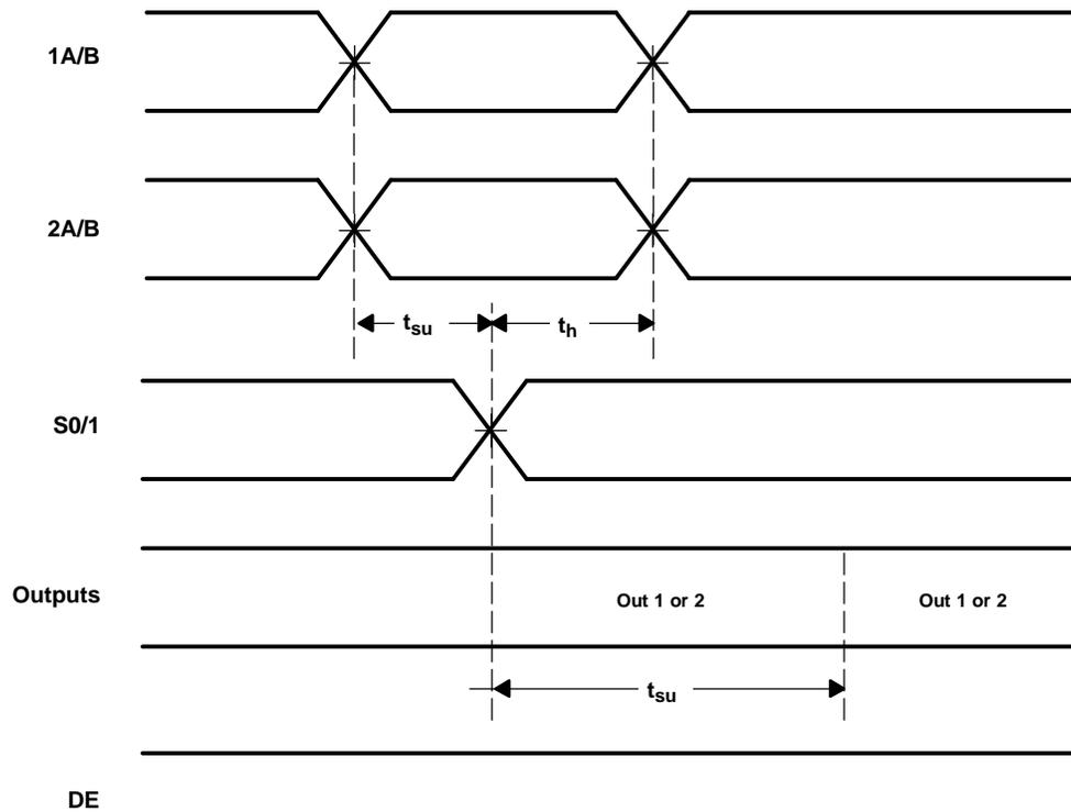
NOTE:  $t_{su}$  and  $t_h$  times specify that data must be in a stable state before and after MUX control switches.
