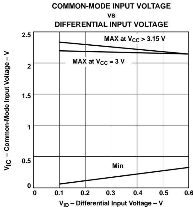
**Figure 1. Common-Mode Input Voltage vs Differential Input Voltage**
