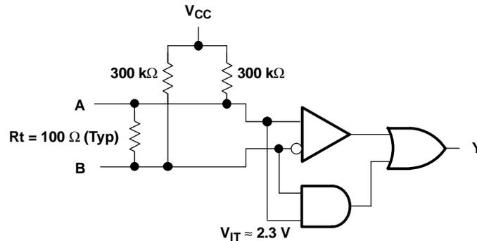
**Figure 11. Open-Circuit Fail Safe of the LVDS Receiver**
