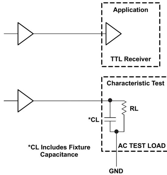
Figure 1. TTL Output Loading Used for Device Evaluation
