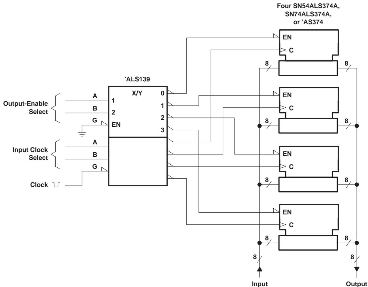
**Figure 1. Expandable 4-Word by 8-Bit General File Register**
