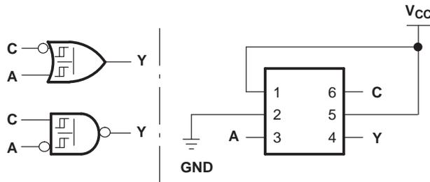
**Figure 7. 14+02/14+08: 2-Input NOR Gate With One Inverted Input**
