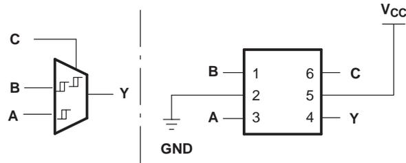
**Figure 5. 157+04: 2-to-1 Data Selector With Inverted Output**
