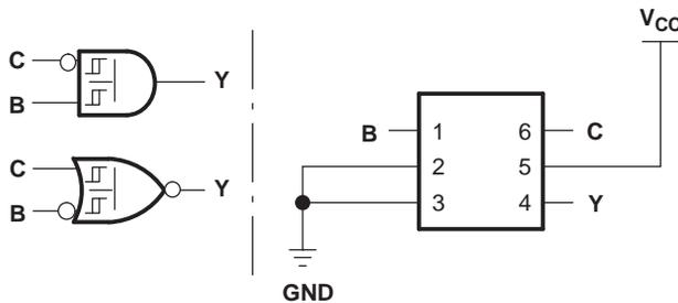
**Figure 8. 14+00/14+32: 2-Input NAND Gate With One Inverted Input**
