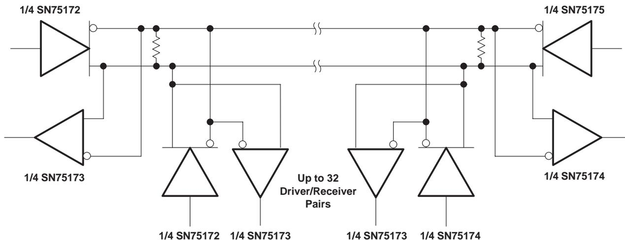
NOTE A: The line should be terminated at both ends in its characteristic impedance. Stub lengths off the main line should be kept as short as possible.
