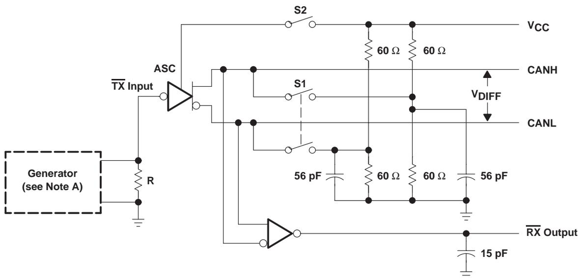
NOTE A: The input pulse is supplied to  $\overline{\text{TX}}$  by a generator having a  $t_r$  and  $t_f = 5\text{ ns}$ .
